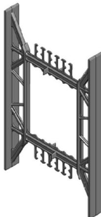
**Figure 2 – Fox Block ICF System Web Connector**
